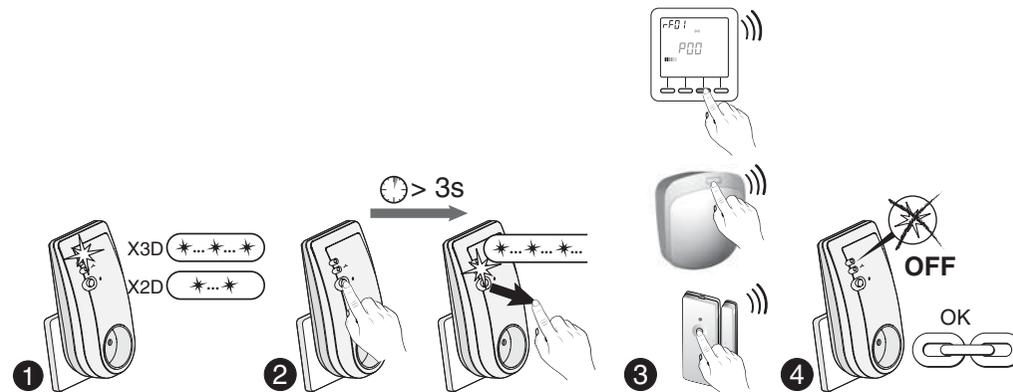
1 When switching on the installation (1) Wait until the LED flashes: 2 times (X2D) or 3 times (X3D).
